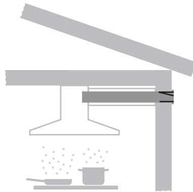
With visible side exhaust duct
