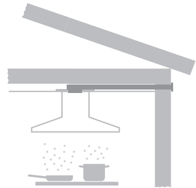
With concealed exhaust duct, e.g. suspended ceiling with flat channel exhaust air conduit
